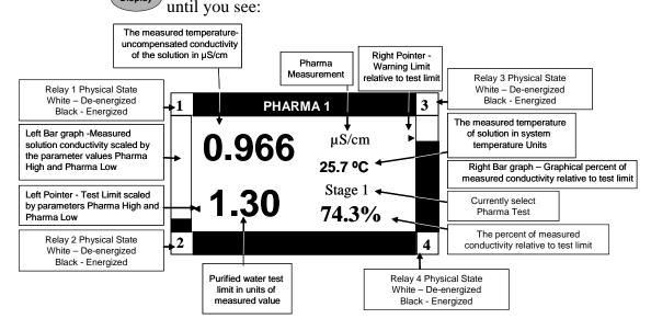
Figure 5-5 Pharma Display screen example
